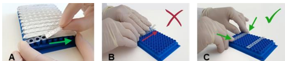
Figure 1: A. Removing foil from PCR strips. B. Incorrect way to close lids in one direction. C. Correct way to close lids by first softly fixing the ends of the cap strip to the reaction tubes, than applying even pressure to tightly close the PCR strips.
