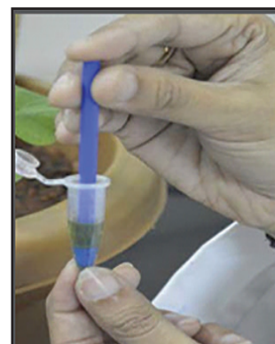
Extracting protein by crushing with pestle
