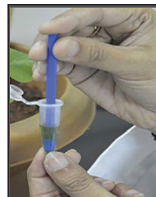
Extracting protein by crushing with pestle
